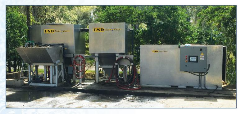
**Solid Managment Systems.** ESD Waste2Water, Inc offers a system to eliminate large in-ground sumps and drive-in pits saving on space and messy clean outs. The Solids Management System (SMS) is designed to handle solids above ground while recycling the wash water. The SMS is designed to process large amounts of sludge and place into an easy to remove Solids Hopper. The models 700 & 800 Systems will reduce operator maintenance for heavy wash applications such as:
