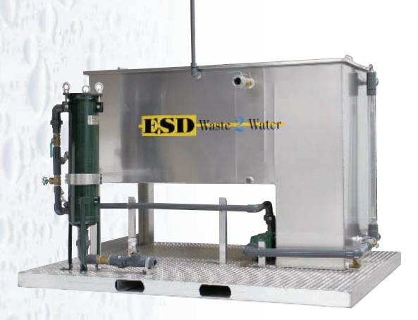
**ESD** Waste Water, Inc. manufactures a complete line of above ground corrugated plate enhanced oil/water separators. The separators are designed to remove free and dispersed non-emulsified oil and settable solids in accordance with API 421.
